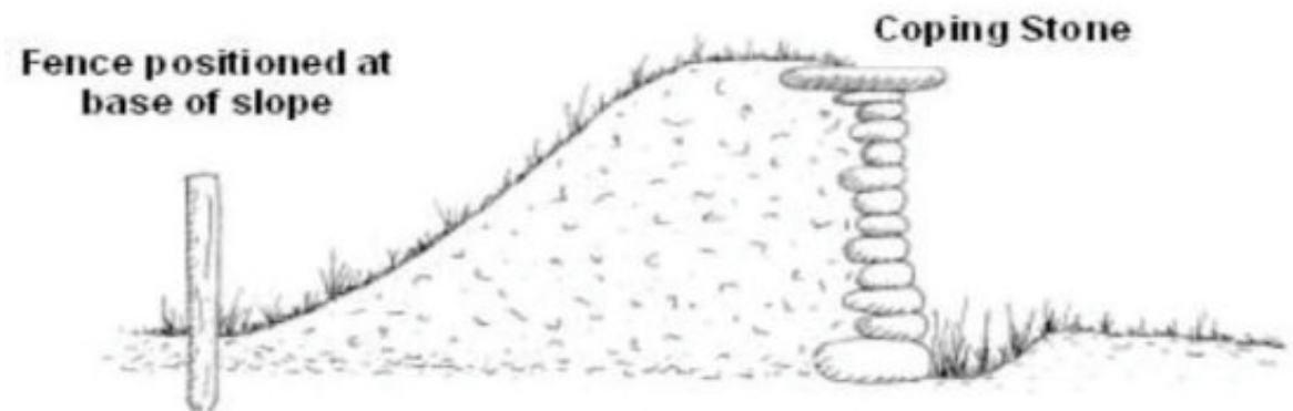
Fig. 2. Section through a typical corn ditch.
